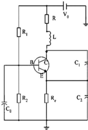
Fig. 1. Circuit diagram of the chaotic Colpitts oscillator [7]
