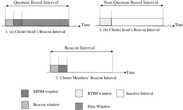
Fig. 5. Structure of beacon intervals, 1: (a) & (b) for cluster heads, 2: for cluster members
