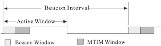
Fig. 2. Structure of a BI in the quorum interval
