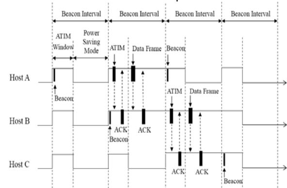
Fig. 1. Structure of IEEE 802-11 PSM
