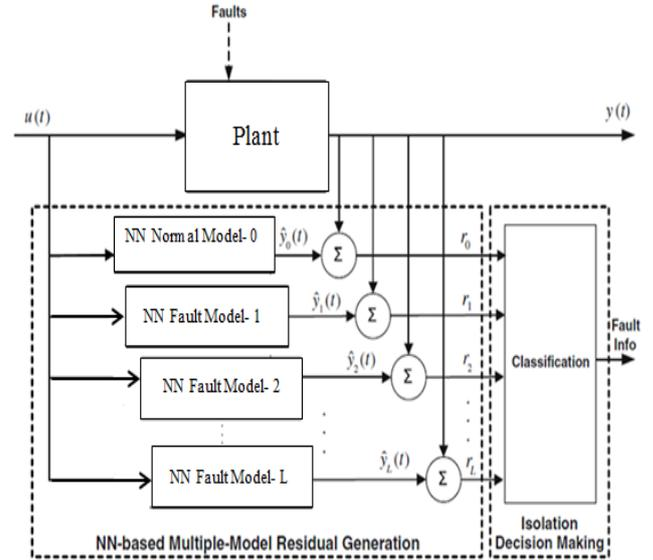
Fig. 3. General method of fault detection and isolation, neural network-based multiple model [17]
