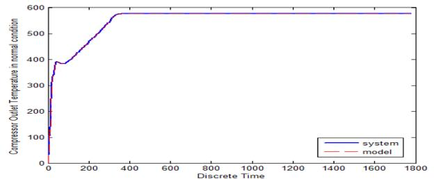
Fig. 5. LLNF model performance for Compressor Outlet Temperature
