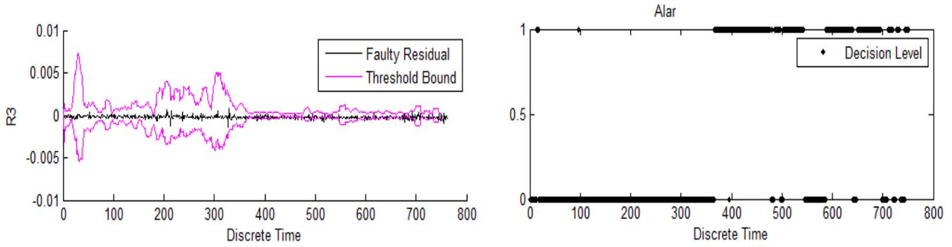
Fig. 16. Fault detection using adaptive threshold and decision making for  $f_3$  using Combustion Chamber Outlet Pressure
