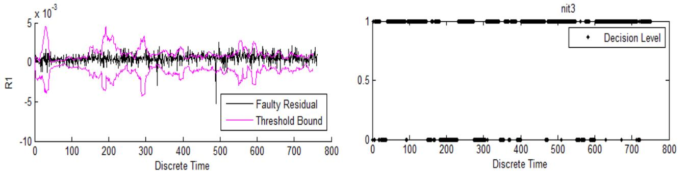
Fig. 14. Fault detection using adaptive threshold and decision making for  $f_1$  using Compressor Torque
