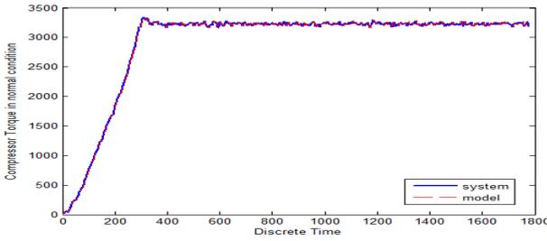
Fig. 6. LLNF model performance for Compressor Torque
