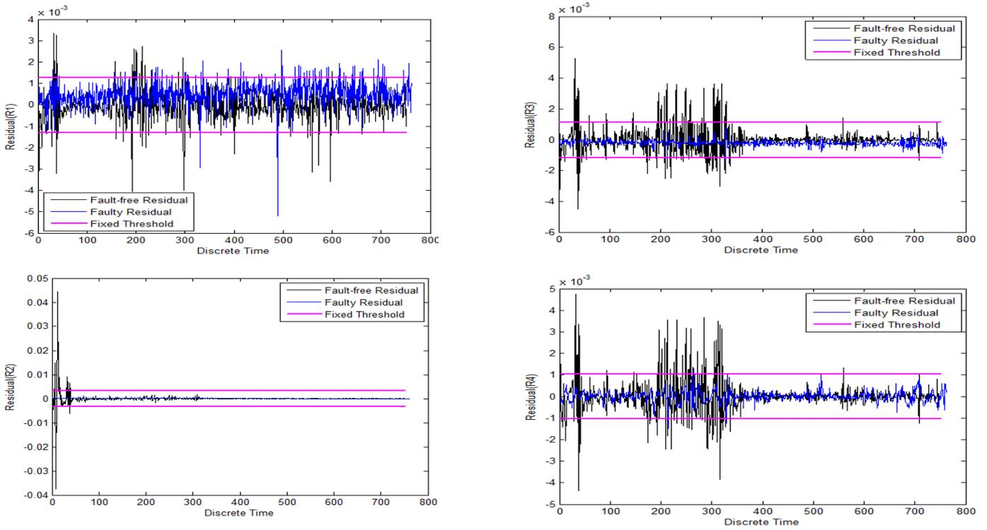
Fig. 13. Generated residuals and constant threshold in the test phase for  $f_1, f_2, f_3, f_4$
