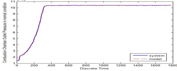
Fig. 7. LLNF model performance for Combustion Chamber Outlet Pressure
