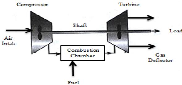
Fig. 2. The simple-cycle gas turbine block diagram [7]
