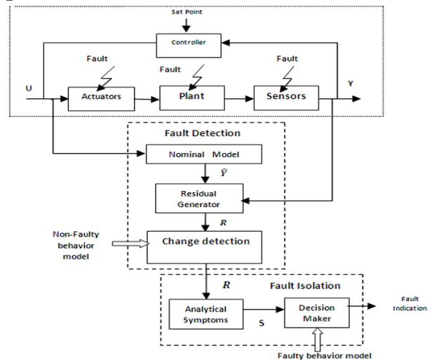
Fig. 1. General scheme of fault detection and isolation [10]
