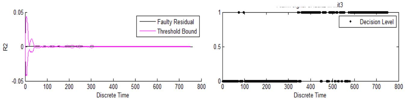
Fig. 15. Fault detection using adaptive threshold and decision making for  $f_2$  using Compressor Outlet Temperature
