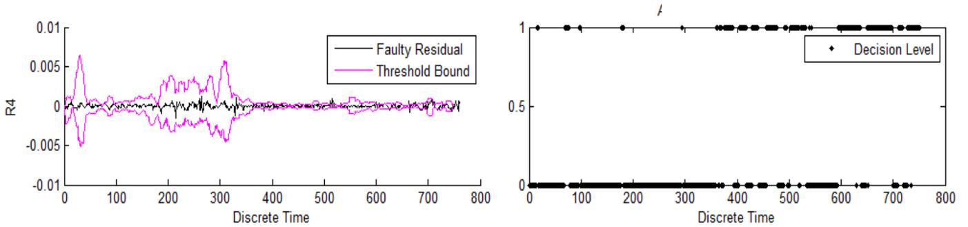
Fig. 17. Fault detection using adaptive threshold and decision making for  $f_4$  using Compressor Inlet Pressure
