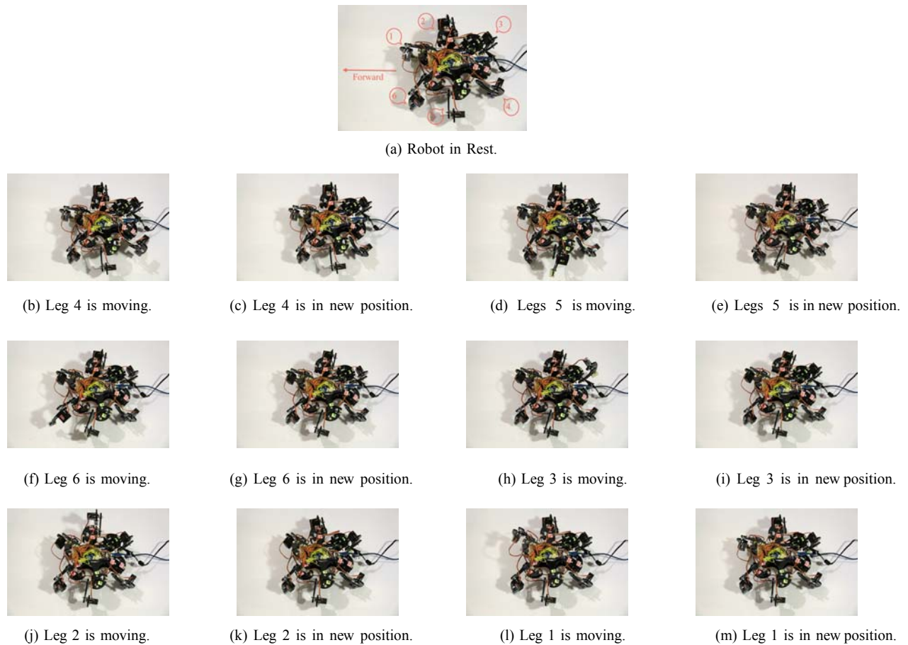
Fig. 6. Wave gait implementation on SiWaReL prototype in one step
