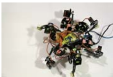
(b) Legs 1, 3 and 5 are moving into new position.
