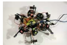
(h) Legs 2, 4 and 6 are moving into new position.
