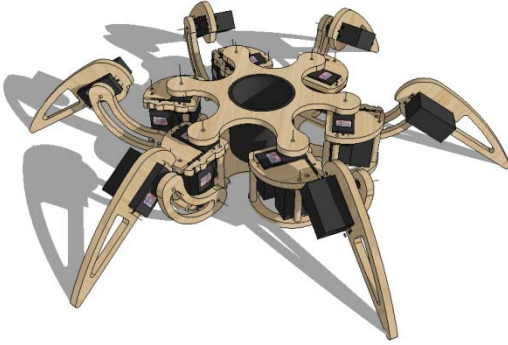
Fig. 2. 3D model of 18 DoF SKPRbot hexapod
