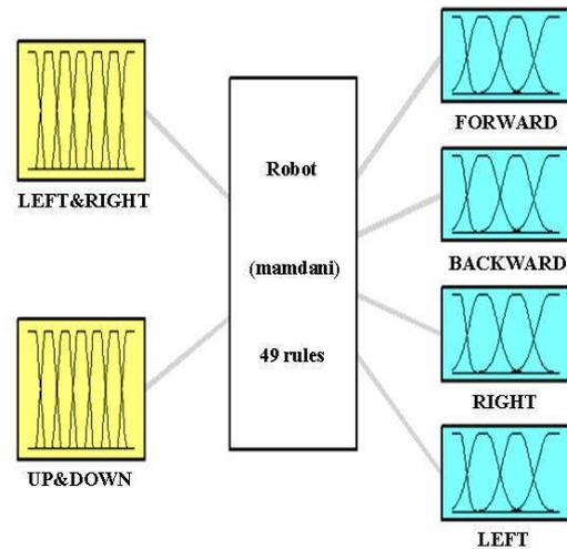
Fig. 4. Fuzzy system input and output structure.
