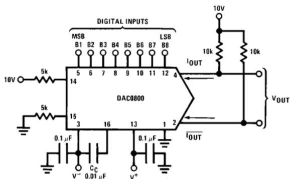
Fig. 2. Driver circuit DAC0800 with amplified output.
