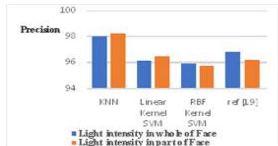
Fig. 14. The results obtained from comparing identification rate for three classifiers in ORL database
