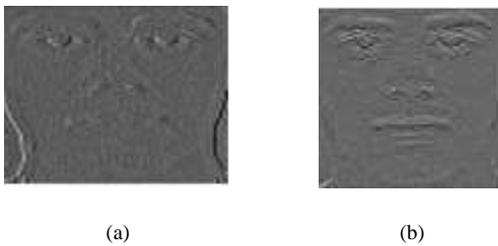
Fig. 6. The imaged obtained by Gradient of the two Sobel kernels (a. vertical gradient kernel, b. horizontal gradient kernel)
