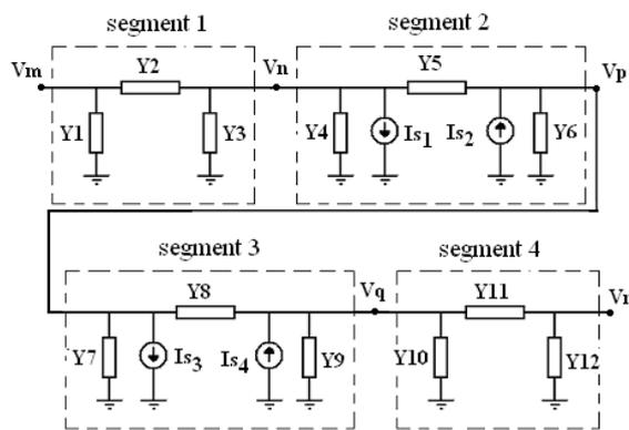
Fig. 10 Pipeline equivalent circuit.
