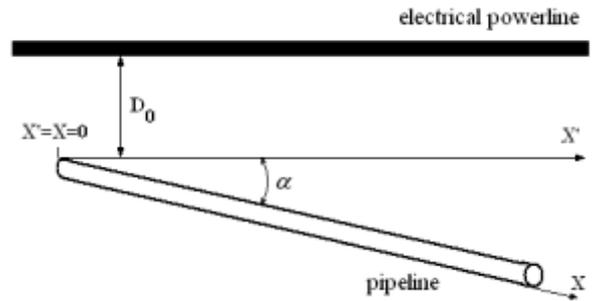
Fig. 6 Ramped pipeline relative to power line
