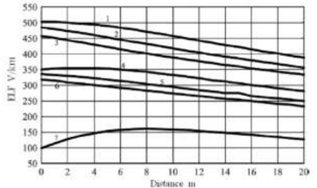
Fig.1 LEF as a function of distance in various faults to the ground, 1: phase c to ground, 2: phase b to ground, 3: phase a to ground, 4: phases a & c to ground, 5: phases a & b to ground, 6: phases b & c to ground, 7: phases a & b & c to ground.
