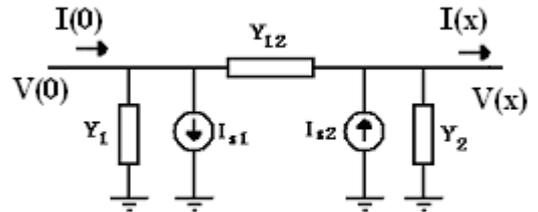
Fig. 4 Two ports  $\pi$  model circuitry for the parallel pipeline
