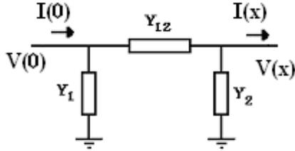
Fig. 7 Two ports  $\pi$  model circuitry for the orthogonal pipeline
