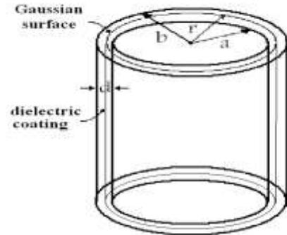
Fig. 8 Pipeline, Gaussian surface and dielectric coating.
