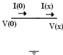
Fig. 5 Simplified model for very small length of pipeline.
