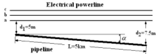
Fig. 11 ramped pipeline.
