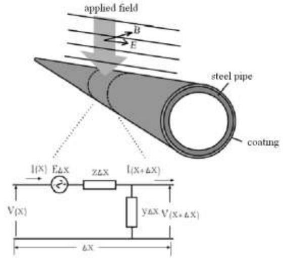
Fig.3 Transmission Line Model (TLM).
