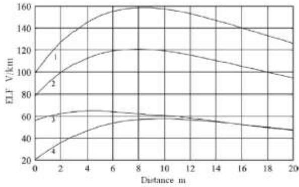
Fig.2 ELF as a function of distance in various phase to phase faults, 1: three phases together, 2: phases b & c, 3: phases a & c, 4: phases a & b.
