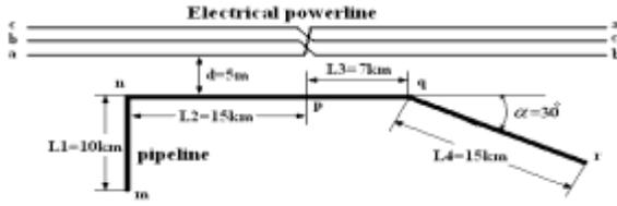
Fig. 9 Power line and adjacent pipeline.
