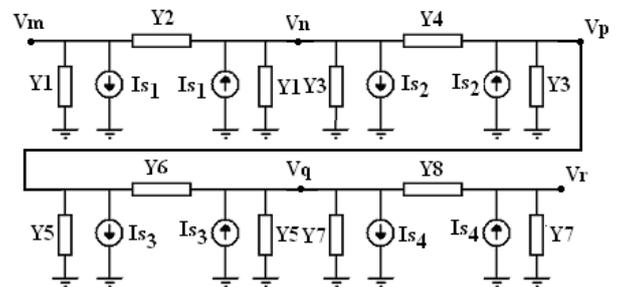
Fig. 12 Equivalent circuit of ramped pipeline
