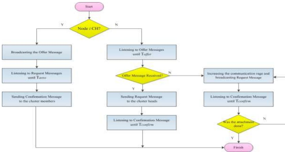
Fig. 6. Flowchart of attachment of member sensor nodes to the corresponding cluster head.
