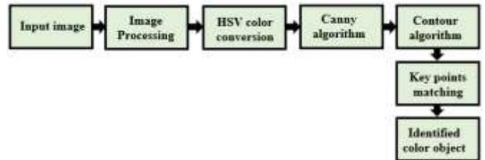
Fig. 3. Diagram Block Diagnosis and Identification of window
