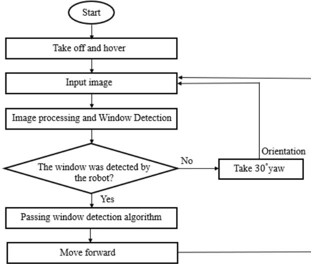
Fig. 5. Flowchart of the proposed algorithm for passing the error position window
