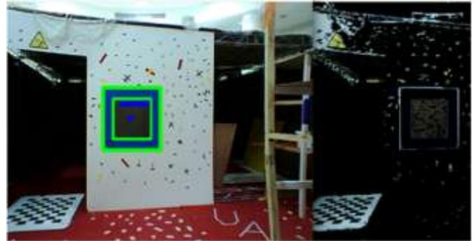
Fig. 10. Indoor window identification using a quadrotor Bebop2
