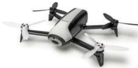
Fig.1. Bebop2 quadcopter equipped with visual navigation system [18]
