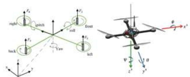
Fig. 2. Quadrotor structure
