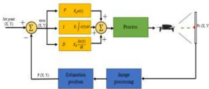
Fig. 8. Closed-loop controller block of the window detection system
