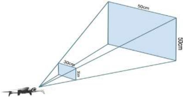
Fig. 11. How to identify a smaller window as an obstacle indoors
