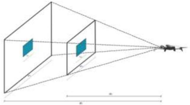
Fig. 7. Angle of view of Parrot Bebop2 quadcopter [7]
