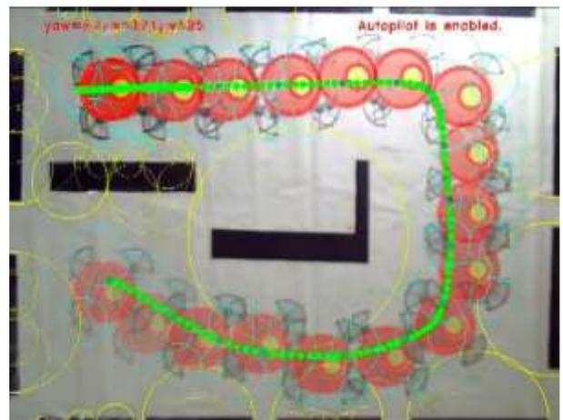
Fig. 11. The quadrotor movement during the tracking experiment which is labeled Test1 in Figure (10).
