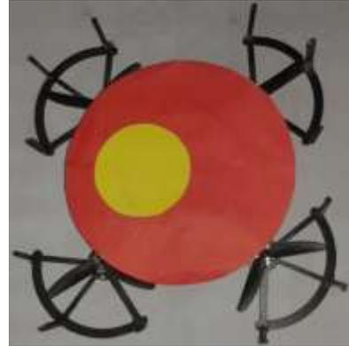
Fig. 4. Two disks are installed on the top of quadrotor to determine the position and angle of the robot.
