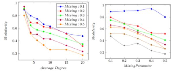
Fig. 6. Impact of the average degree and mixing parameter on the modularity
