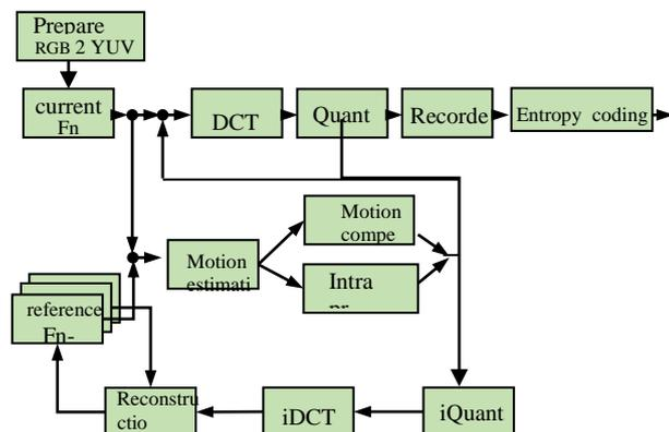
Fig.1.: Encoding diagram in HEVC video standard [14].
