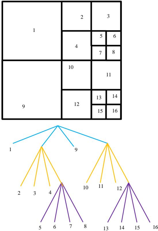
Fig.2. An example of division of one CTU to encoding blocks.
